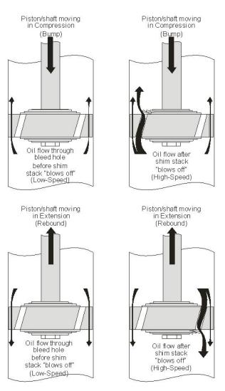
Most good racing/performance shocks today allow you to adjust the Bump without affecting the Rebound, and vice versa. As well, you should be able to change the High-Speed characteristics without affecting the Low-Speed, and vice versa. With less expensive shocks, or ones not made for the track, you can't do this. Obviously, to get the full potential from your car, you need to be able to adjust specific characteristics of the shock without affecting others.
