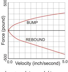
A linear characteristic means the damping force increases at the same rate as the piston speed. Progressive means the damping force increases at a greater rate than the increase in piston speed. And, digressive means the damping force increases at a lesser rate than the increase in piston speed.
