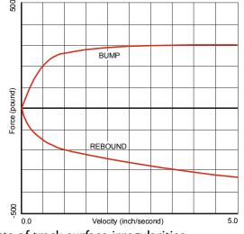
Sometimes, a car feels as though it is rolling too much at either the front or the rear. If that's the case, increase the Low-Speed Rebound at that end.
