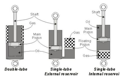
the force required for the oil to open them and allow the flow through that particular orifice. The overall combination of the size and layout of the orifices in the piston, along with shims covering the holes, determines the force developed by the shock, and therefore the characteristics of the shock.
