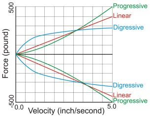
Through careful use of various piston shapes, orifices layouts and sizes, and shims, a combination of linear, progressive and/or digressive can be achieved. For example, the curve can start out being linear, and then change to digressive; or, start out progressive and then change to digressive. It's all a matter of what you what the shock to do.
